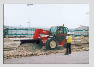
It also has a wide digging angle making it easy to pick up and tip building materials. It is also the ideal tool for clearing building sites.
